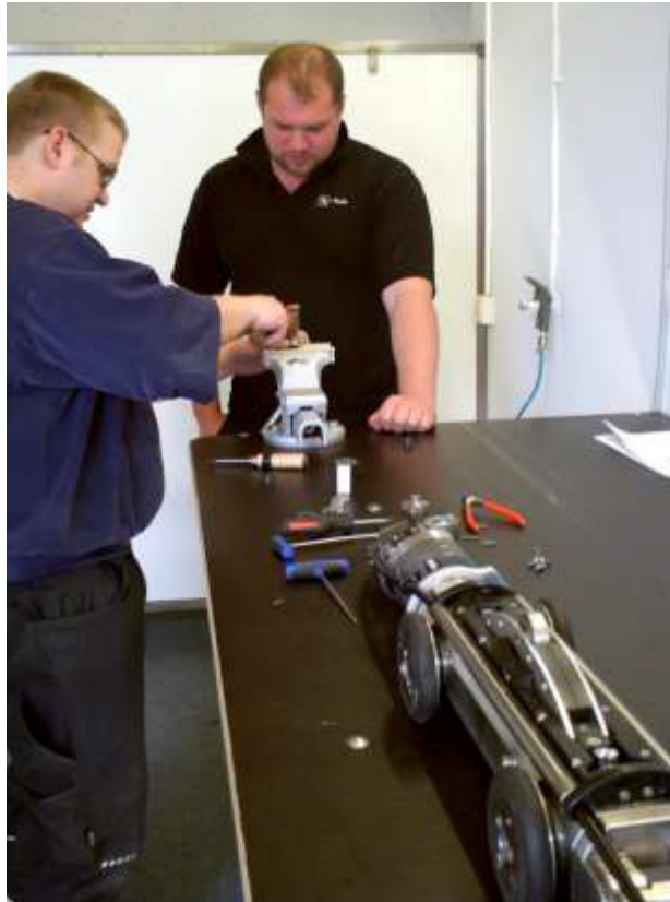
Maintenance work on an IBG HydroCut milling robot.
